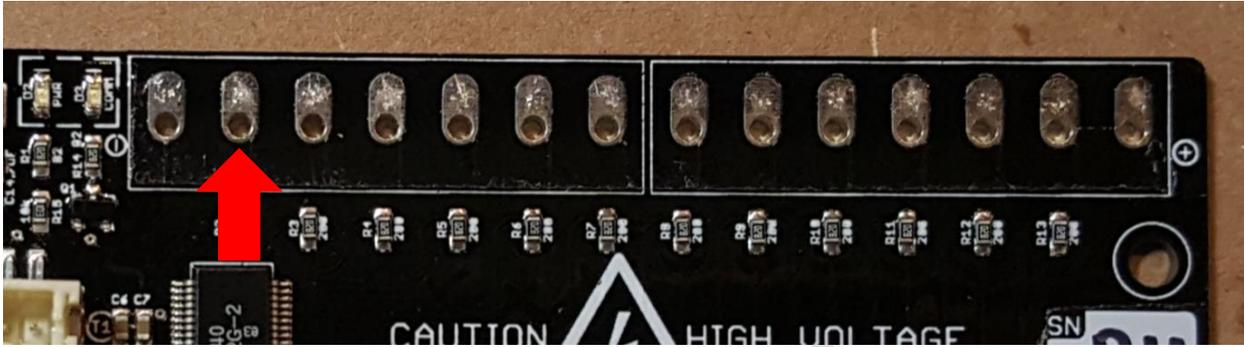
Continue this process until you have connected all sense lines, or have reached the 13 line limit of a single board.
