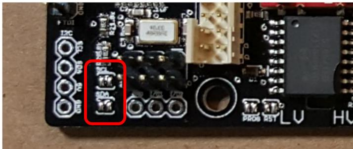
If your bus already has pull up resistors, these can be disabled by cutting the thin trace between them on the top side of the board with a sharp hobby knife. They can also be re-enabled by jumping the pads again with solder.
