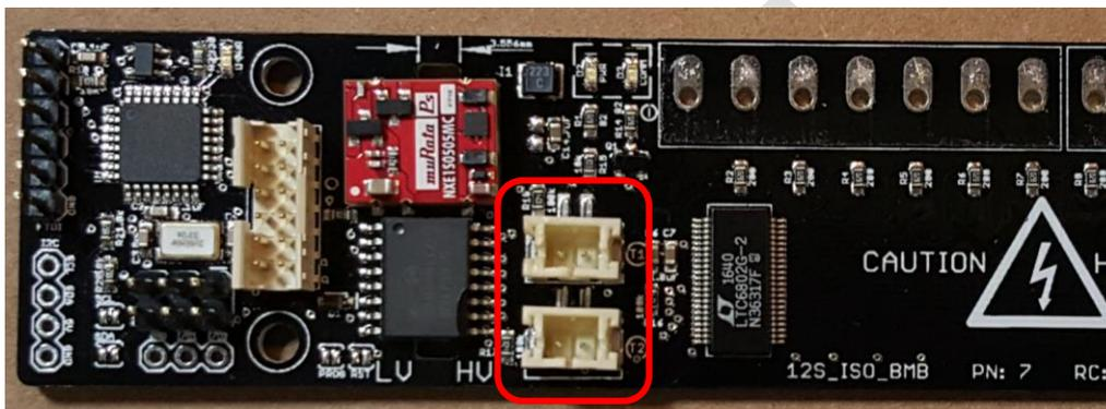
Many pre-terminated thermistors are available online. The only requirement for your chosen thermistors is that they have a nominal 100kOhm resistance, and that they will operate in a useful temperature range for your battery. Basic thermistor lookup tables are provided for the following commercial thermistors in the four-forty BMB codebase:
