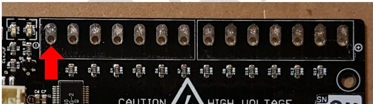
Now proceed to the next potential voltage sense line, which should be connected to the next series cell in the stack.
