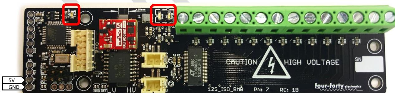
The board is **not** protected against reverse polarity hook-ups, so check the wiring twice! If the board is being powered successfully, you should see 3 LEDs turn on in the above locations (lights may blink or go out after startup, this is normal).
