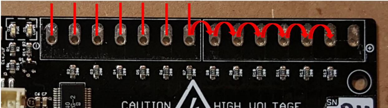
If you plan to monitor more than 12S, you'll need to split your sense lines between multiple boards. This also means that sense line number 13 will be top of stack on your first board, and bottom of stack on the second. To accommodate this, use the 14<sup>th</sup> position to run a wire jumper to the negative-most position on the next board.
